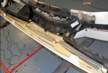
Also take down the polyurethane vibration-damper support.
