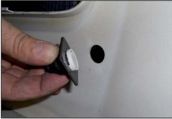
Near the sensors measurement, drill a hole in the rear plastic support using a 35 mm mill.
