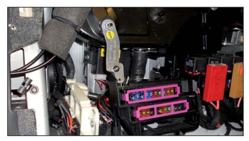
The front management control unit and the CAN BUS utility module must be set up over the GFA control unit located under the glove compartment, on the passenger's side.
