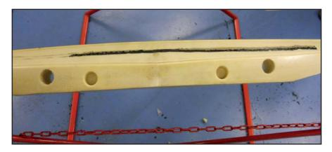
Near the sensors measurement, drill a hole in the vibration-damper support using a 35 mm mill.
